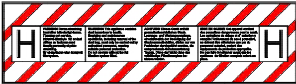
Figure AA.1 – Warning label for dust class H machines
